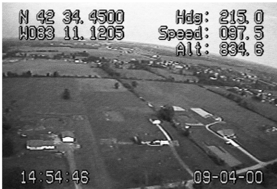
Fig 1.0 - Screen shot of OSD-GPS on a rocket.
